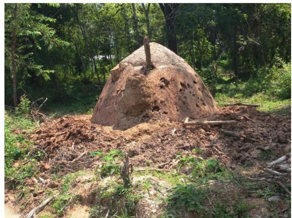
**Figure 3** Termite mound for charcoal kiln. Base diameter and height of kiln were 2.4 m and 1.8 m, respectively. Termite species was unknown.
