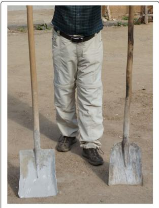
**Fig. 4** Two spade handles – the one on the left made from *Meliosma* wood, the one on the right from *C. kousa*
